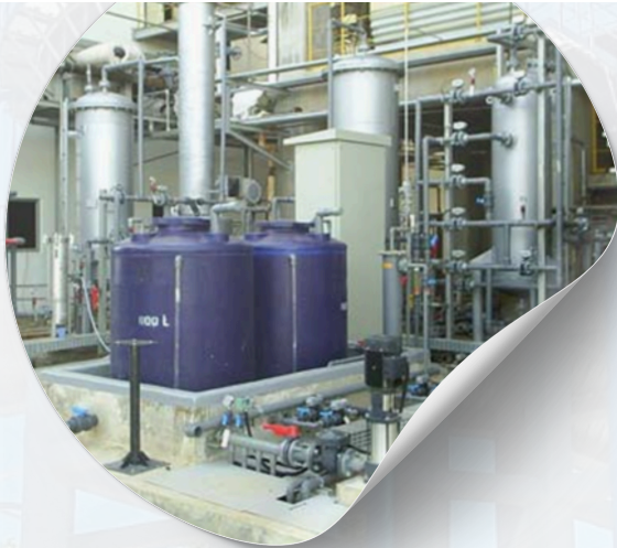
Demineralized & Mixed Bed Water Plant, Capacity : 12 m 3 /h
